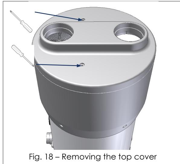
Fig. 18 – Removing the top cover
