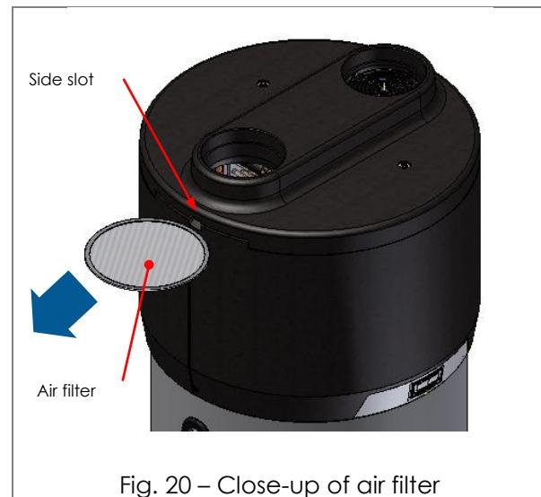
Fig. 20 – Close-up of air filter
